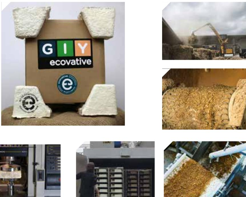
**Figure 4.5** Production of Mycofoam™ from agricultural waste, showing the raw material, inoculation by a fungal strain, incubation and pressing. The example shows protective corner mounts, replacing the use of EPS; images courtesy of Ecovative.
